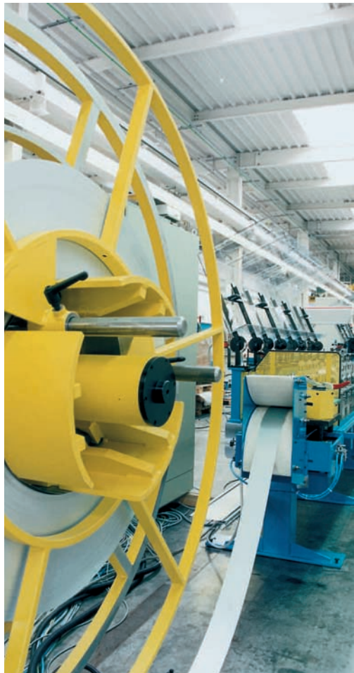
uncoiler with pneumatically activated disc brake
