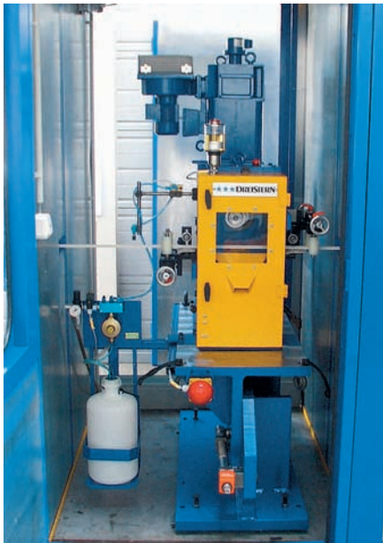
light-slot punch unit (twin-cam unit) with sound proofing enclosure
