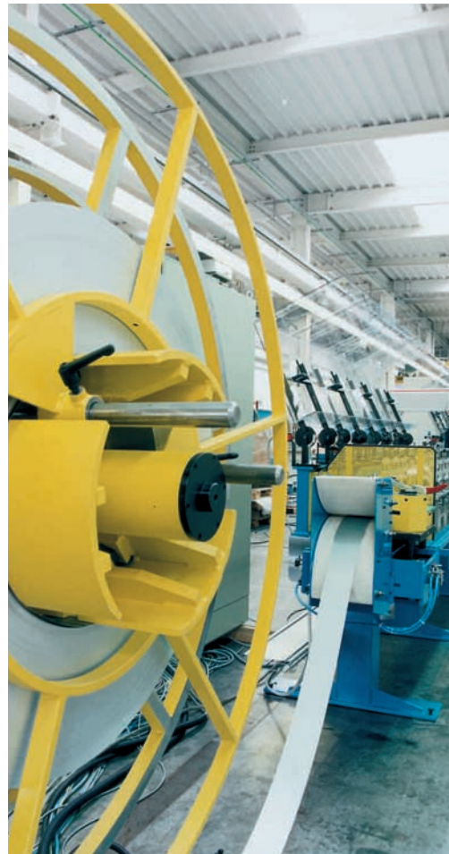
uncoiler with pneumatically activated disc brake
