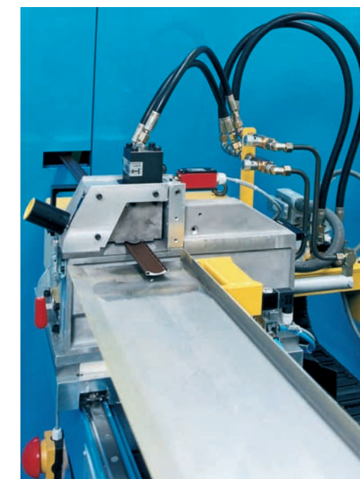
flying high speed cut-off saw unit with run-out table
